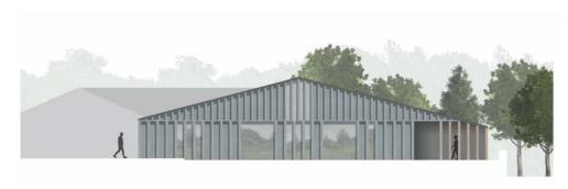
SOUTH ELEVATIONAL TREATMENT OF OVERCLAD RENDERED WALLS TO PORTAL FRAME
